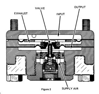
(Invensys An Invensys company A further increase in the input pressure will cause the lower portion of the valve to open until the output pressure again equals the input pressure. A decrease in input pressure will allow the output pressure to force the center assembly upward, opening the exhaust valve until the output pressure is equal to the input pressure.
